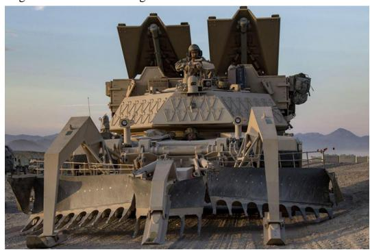
The Assault Breacher Vehicle (ABV) is a tracked armored engineer vehicle specifically designed for conducting instride breaching of minefields and complex obstacles. The ABV is built on the same chassis as the General Dynamicsbuilt M1A1 Abrams main battle tank. The Assault **Breacher Vehicle** (ABV) is a single
