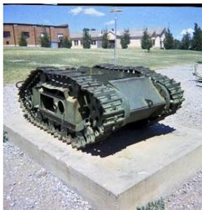
(Goliath Light Charge Carrier) was a name given to two German Unmanned ground vehicles, disposable demolition vehicles, used during World War II. These were the electrically powered *Sd.Kfz. 302* and the petrol-engine powered *Sd.Kfz. 303a* and *303b*. They were known as *beetle tanks* to the Allies.
