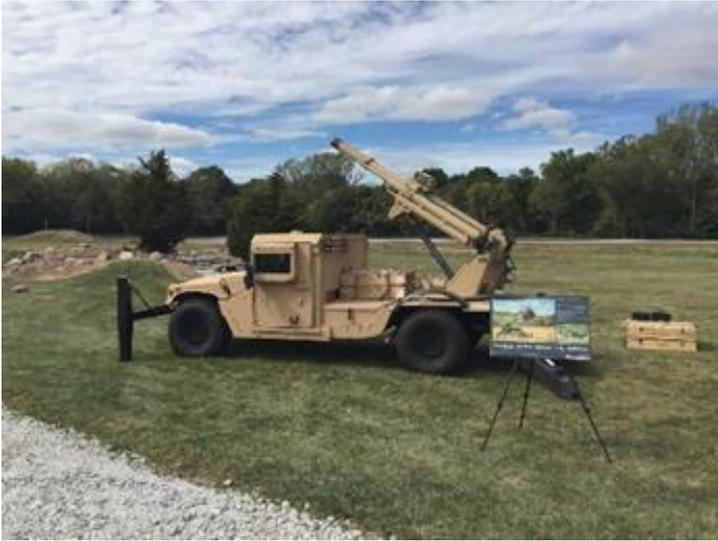
*The Hawkeye, a 105mm artillery piece mounted on a Humvee by AM General, using Mandus Group's "soft recoil" technology, makes for a more mobile, transportable artillery piece. (Todd South/Staff)*
