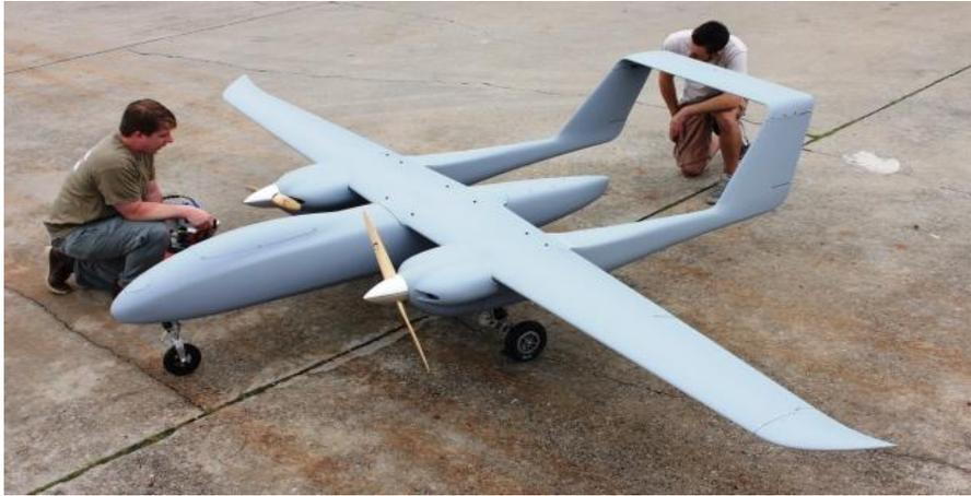
*Example of a SeaHunter unmanned aerial vehicle that was tested in Alma, Que., last month. The device is made by Griffon Aerospace, of Madison, Ala. (Griffon Aerospace)*
